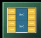
CoWoS (SoC) 3.3-ret., 8x HBM 80x80mm substrate
