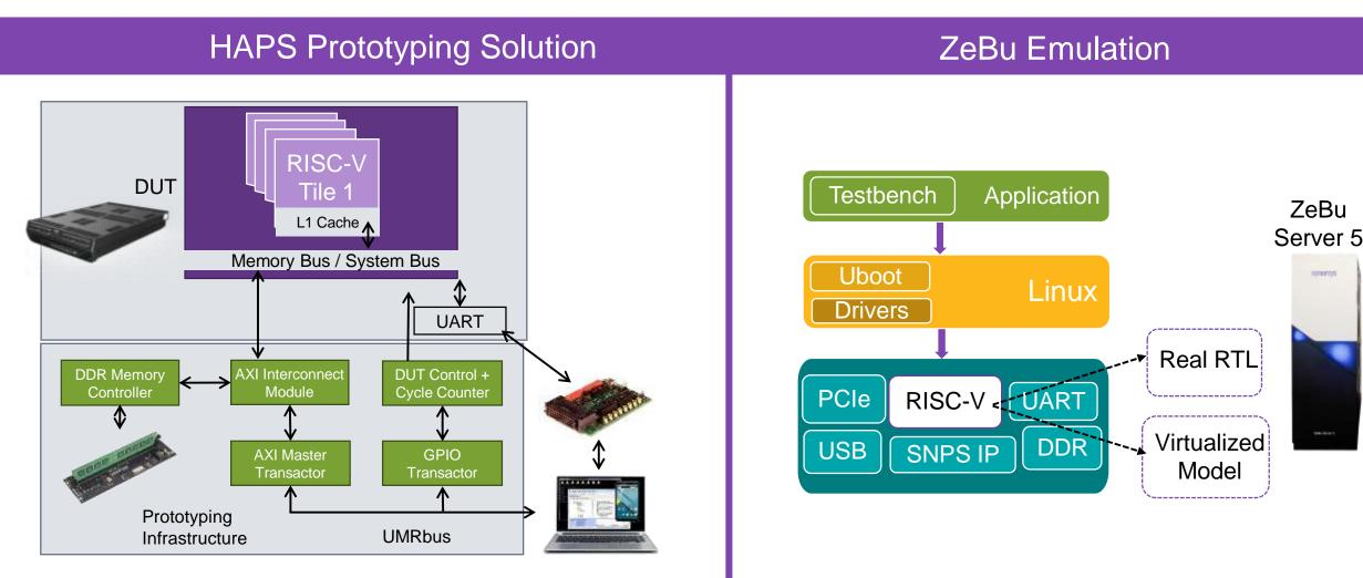
HW/SW debug with real ASIC | Unified RTL debug with Verdi | 4 RISC-V embedded cores running at 100MHz in one FPGA
