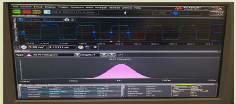
Figure 5: Jitter/Noise Measurement after daughter card installation
