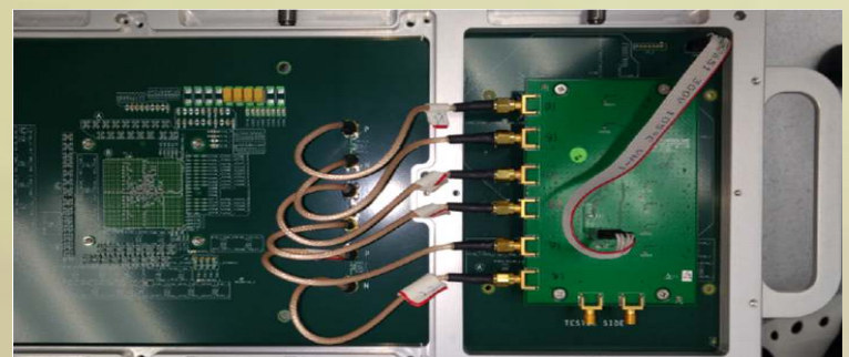
Figure 6: Daughter Card after final installation to ATE HW
