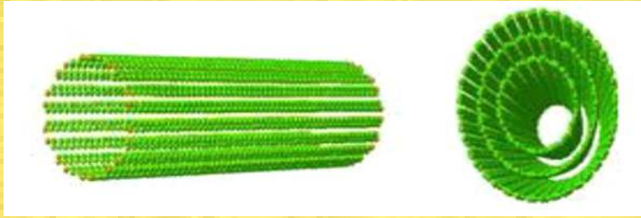
Figure 2: Single walled and multi walled nanotubes (courtesy: http://cnanotubes.blogspot.in/ )
